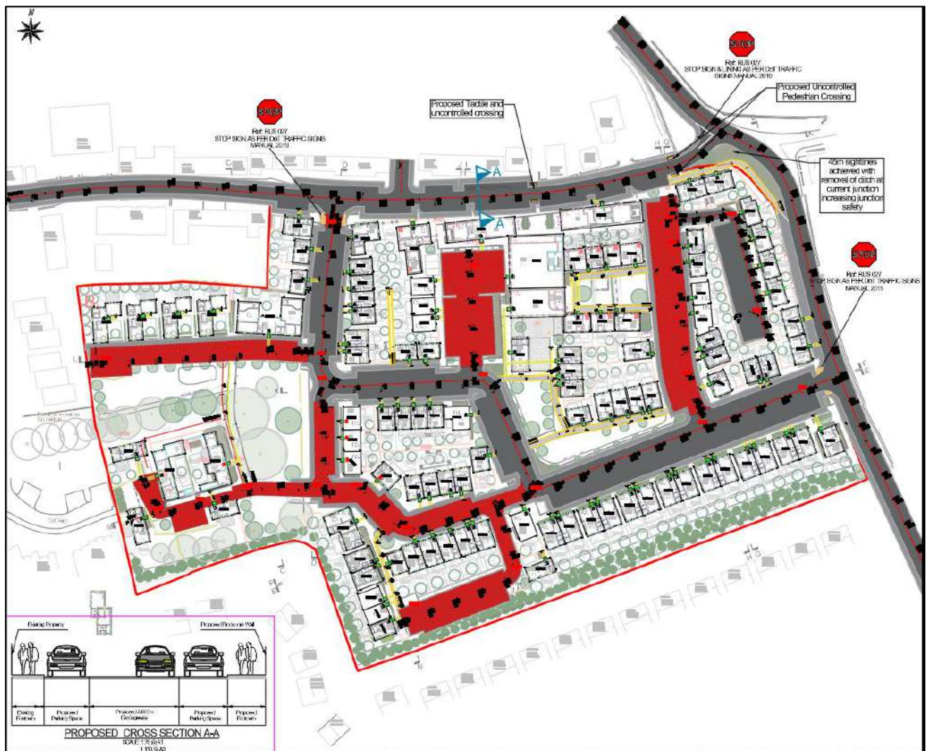
Figure 3.1: Traffic Calming & Pedestrian Connectivity
