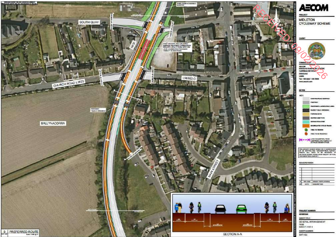
Figure 3.2: Proposed Pedestrian/Cycle Connectivity Improvement Measures along the L96302
